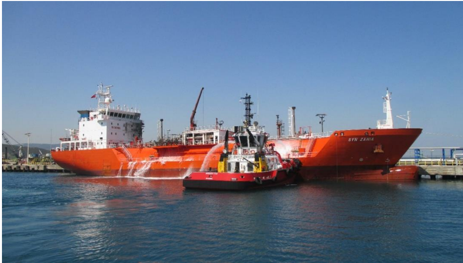
Figure 18: A Snapshot of Cooling Operations
