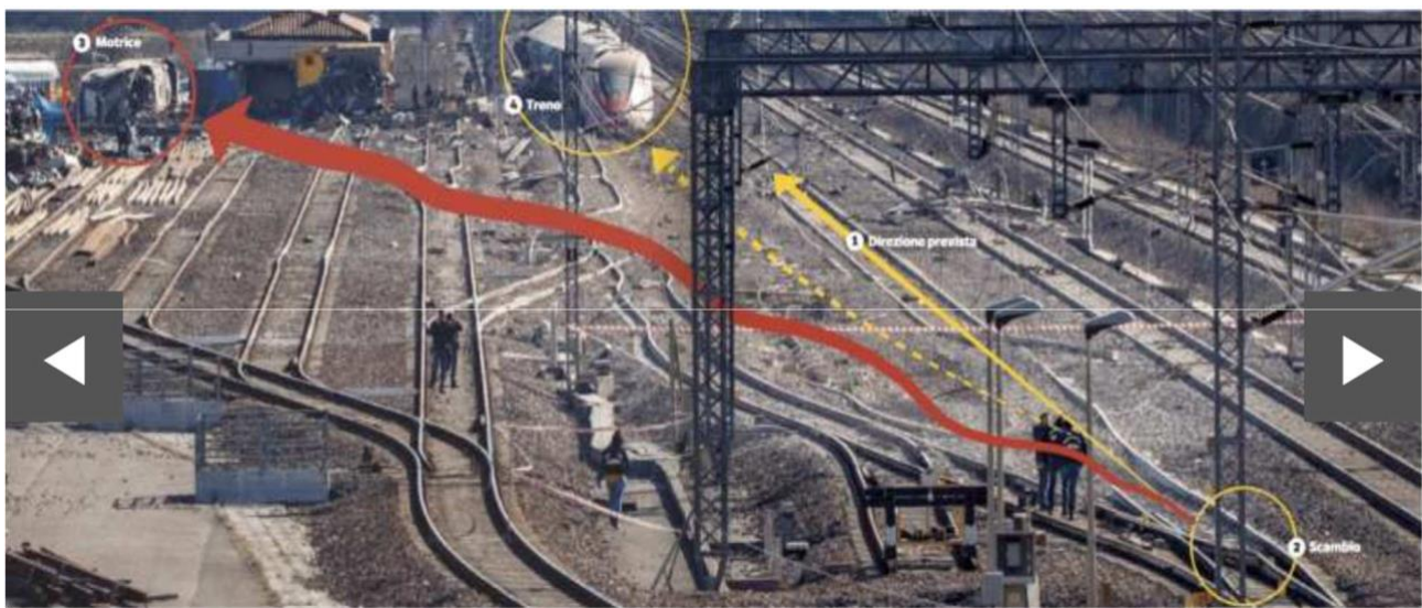
Figure 2 – Schematic reconstruction of the dynamics of the accident (source: web)
