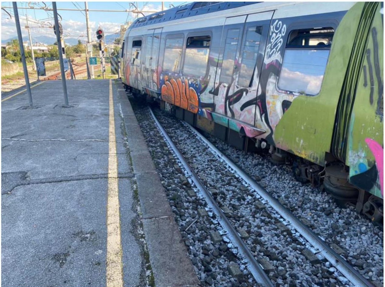
Figure 9 - ETR 208 after derailment (source: EAV).
