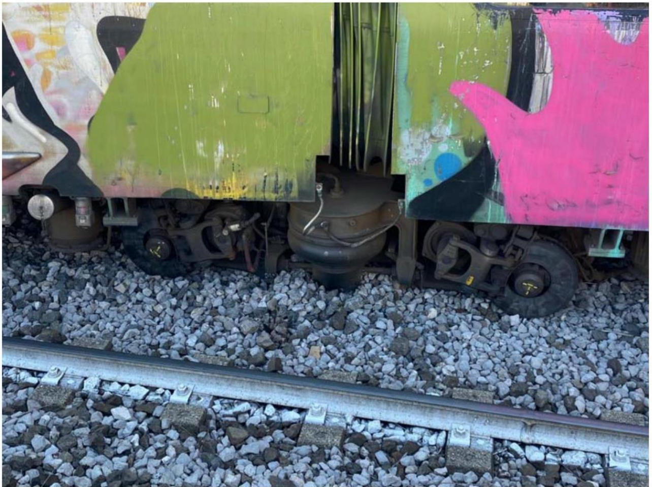
Figure 10 - Bogie no.5 of the ETR 208 after derailment (source: EAV).
