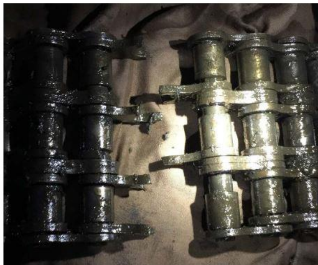
Figure 4: Photo showing the breakage position of main drive chain
