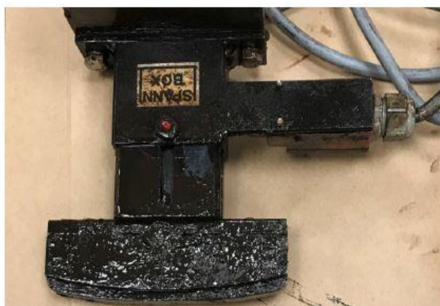
Figure 9: Photo of the BCD moving part and the shoe. Mixture of lubrication oil and dust formed the sticky grease, which was found on the surface.
